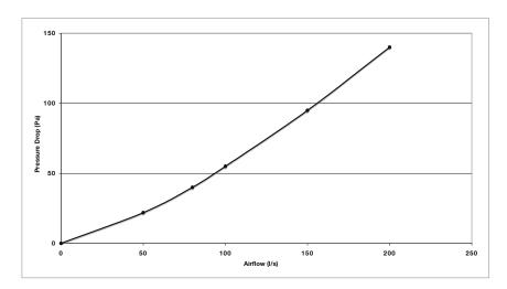
The resistance curve has been constructed from numerical and empirical measurements of the pressure drop across the filter for a range of in-line duct flow rates.
