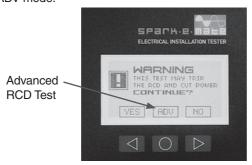
Spark-e-mate briefly displays the ADVANCED RCD TEST mode start up screen.
