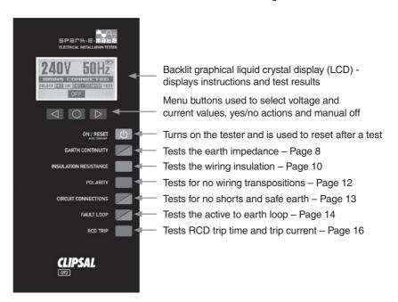
Testing is easily performed from the power point under test simply by plugging the unit in, pressing the ON/RESET button and selecting a test. The LCD then provides an immediate test result.
