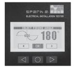
This is the point in the AC waveform that the trip current is applied:
