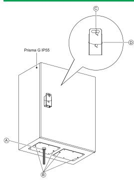
The watt-hour meters comply with the European Measuring Instruments Directive (MID) 2004/22/EC when they are installed in a Prisma G IP55 enclosure (catalog number 08302, 08303, 08304, 08305 or 08306) equipped with a handle padlocking kit (catalog number 08939) in accordance with the instructions prescribed in the EC type-examination certificate summarized below (see diagram opposite):
