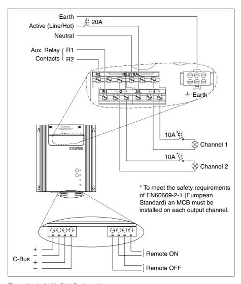
Figure 3 – Lx5102xD10 Series wiring.
