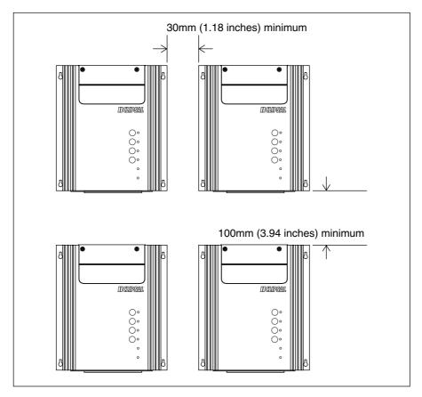
Figure 1 – Mounting clearance for multiple units.
