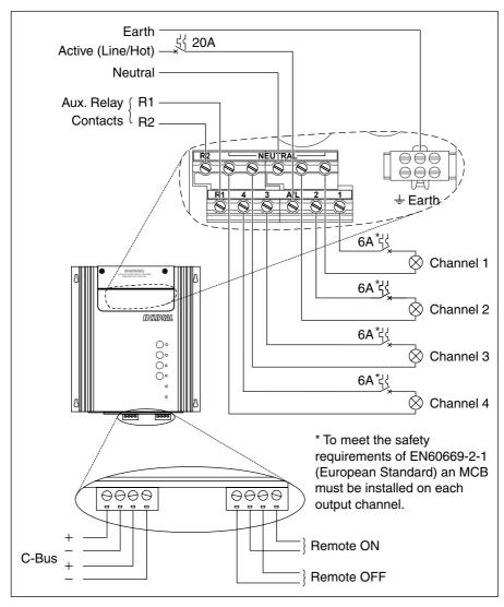
Figure 4 – Lx5104xD5 Series wiring.
