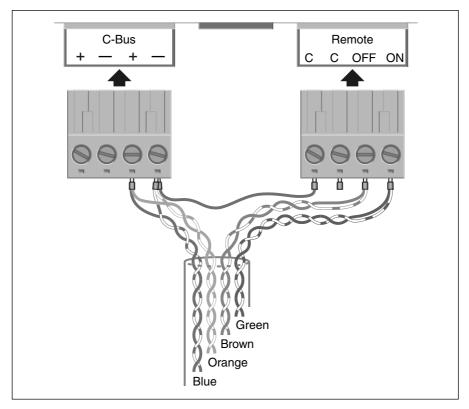
Figure 6 – Standard C-Bus connection with Remote Override connected to C-Bus.
