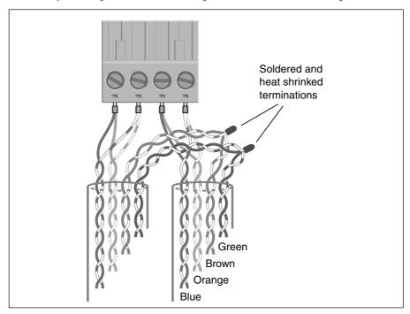
Figure 8 – Daisy-chaining C-Bus cables (maintaining C-Bus Remote Override).
