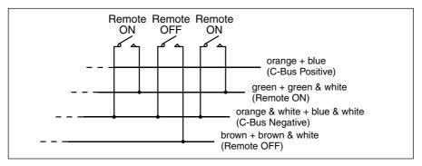
Figure 9 – Remote Override connections.
