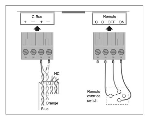
Figure 7 – C-Bus Connection with alternative separate Remote Override.
