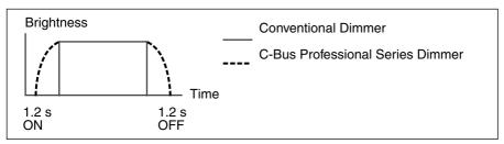
Figure 12 - Channel ON/OFF: Conventional vs C-Bus Professional Dimmer.
