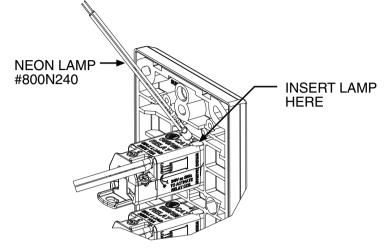
Figure 4: Installation Of Neon Indicator
