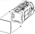
Figure 2: Fitting Front Cover to Relay
