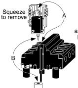
To install fit pins 'A' and 'B' into apertures as shown and press down until the module is locked in place
