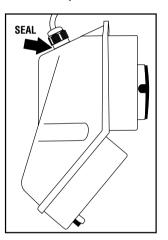
Before fitting bridge apply sealant to slots (see illustration)
