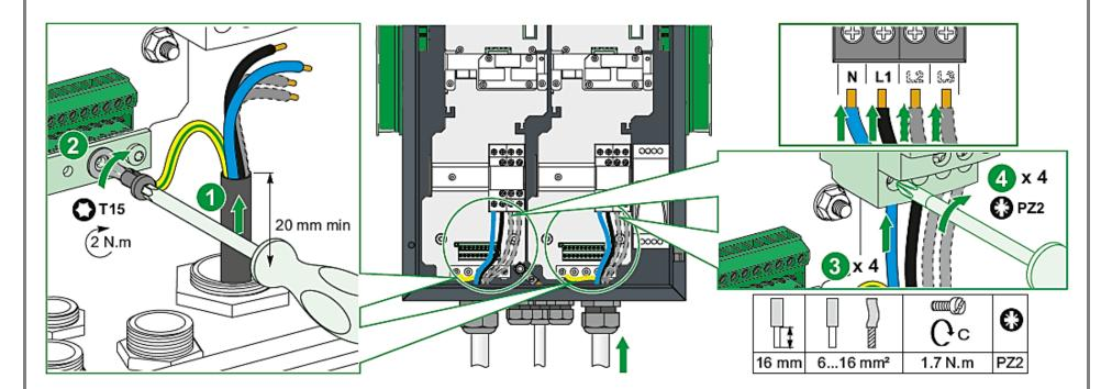
The cable cross-section should be defined by a study to determine the size of the trunking and protection devices. The cables are connected downstream of the contactor.
