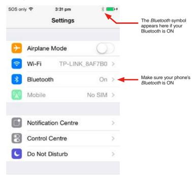
**Important:** Unlike previous *Bluetooth* technologies, the *Bluetooth* Smart module in the *Spark-e-mate* 493BTLi does **not** need to be "paired" with your phone or have PIN codes entered before you can use it. All you need to do is install the Spark-e-log App and make sure your phone's *Bluetooth* is turned on.
