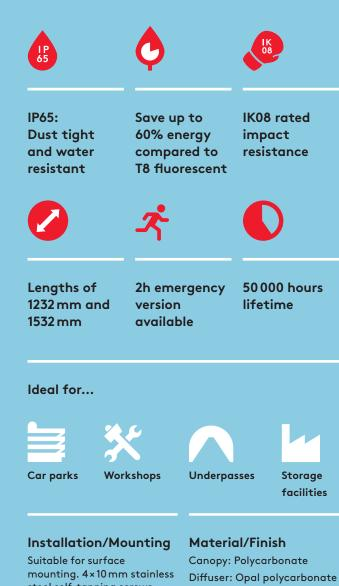
steel self-tapping screws (not included) can be applied to prevent unauthorised opening of the luminaire.
